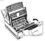
6. Remove the protective foam cylinder from the toner well in the image drum unit.
